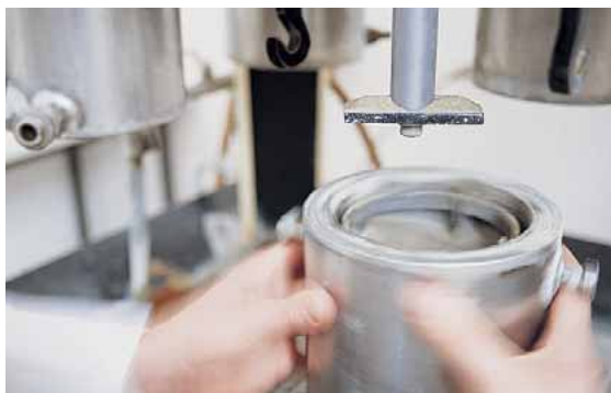
Testing of wear resistance using the sand slurry method is performed regularly in the OKULEN laboratory.
